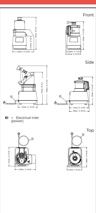
Electric Supply voltage: 220-240 V/1N ph/50/60 Hz **Electrical power max.:** 0.75 kW 0.75 kW **Total Watts:** Capacity: Performance (up to): 150 kg/Cycle Capacity: 2.6 litres Key Information: External dimensions, Width: 348 mm External dimensions, 315 mm Depth: External dimensions, Height: 527 mm **Shipping weight:** 22.2 kg Net weight (kg): 15 **Cold water paste:**
